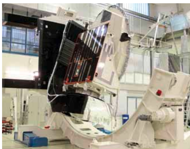
SAR-Lupe satellite during environmental impact testing at IABG in Ottobrunn
