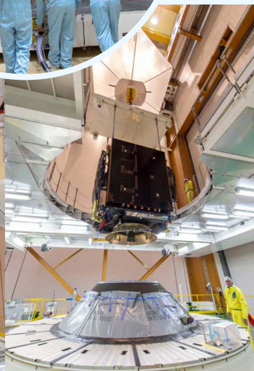
EDRS-C slowly approaching the upper stage of the rocket while hanging from the crane
